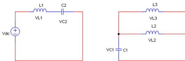
Fig. 3(b). Reduced Equivalent circuit of SL-QZSI under shoot-through state
