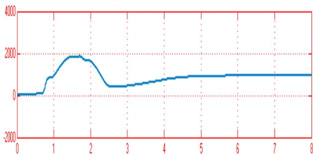
Fig. 26. Motor speed of SIQZSI fed IM with FOPID controller
