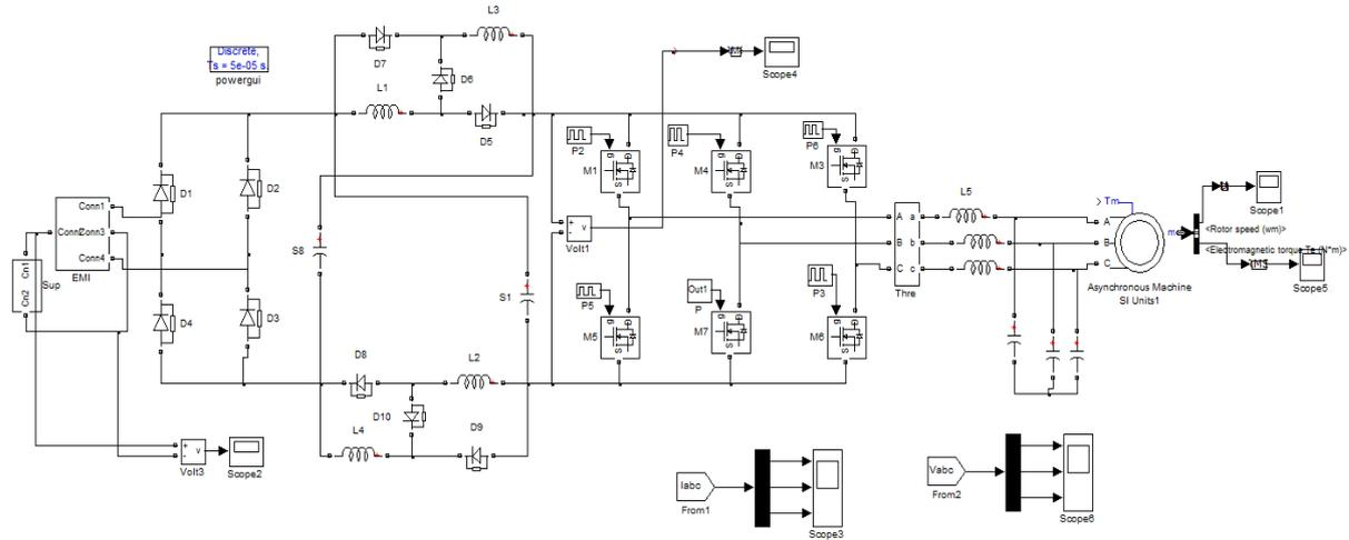
Fig. 7. Simulation diagram of open loop SIQZSI-IM with disturbance
