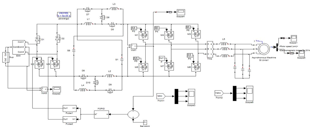
Fig. 21. Simulation diagram of Closed control loop SIQZSI-IM with FOPID controller
