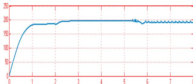
Fig. 16. Voltage across switched inductor quasi Z source of Closed loop SIQZSI fed IM with PI controller
