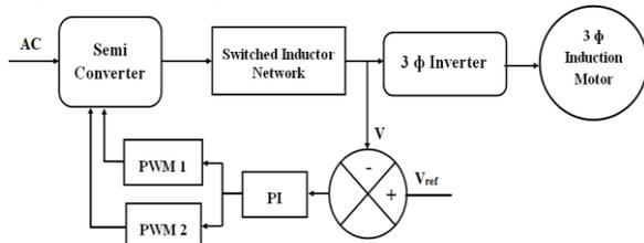
Fig. 5. Block diagram of Closed loop SLQZSI-IM with PI controller
