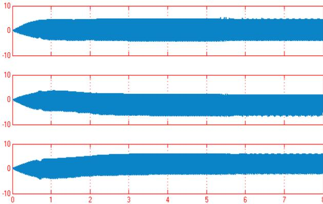
Fig. 18. Current through load of Closed loop SIQZSI fed IM with PI controller
