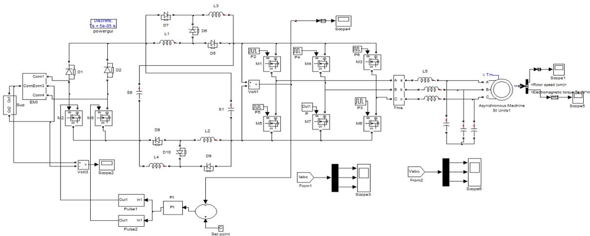
Fig. 14. Simulation diagram of Closed control loop SLQZSI fed IM with PI controller
