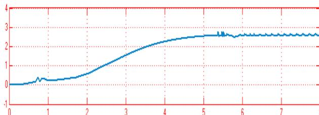
Fig. 20. Motor Torque of Closed loop SIQZSI fed IM with PI controller
