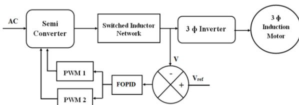
Fig. 6. Block diagram of closed loop SLQZSI-IM with FOPID controller
