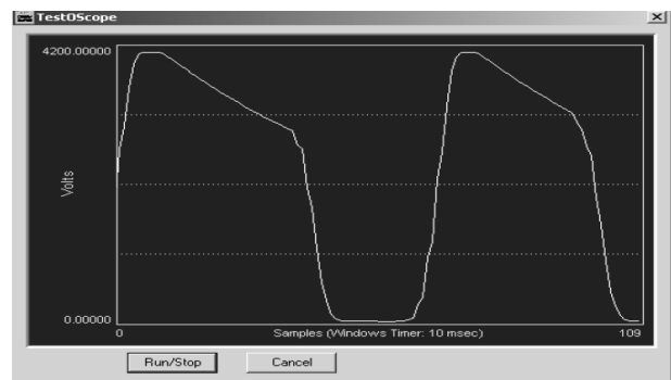
Fig: 6 The response when eyes move up/down
