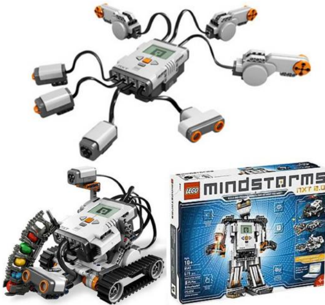
Figure 1. Lego Mindstorms NXT Controller with sensors and a sample mobile robot
