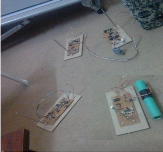
Figure 9: Overall prototype of system with all three sensors and a receiver
