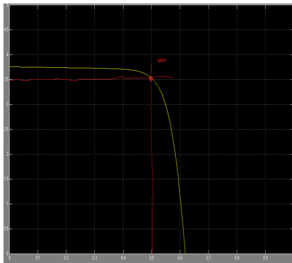
Fig.7. I-V Curve of PV Cell
