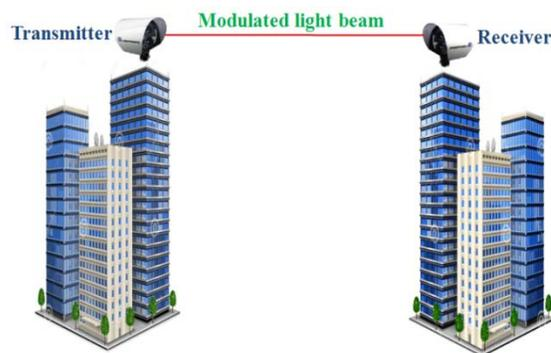
Figure 1: Outdoor FSO link set up on two buildings
