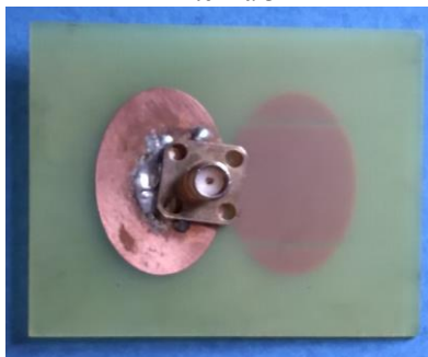
Fig. 2(d): Back view of fabricated antenna structure
