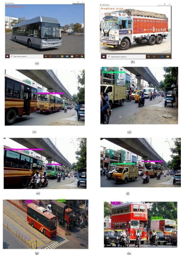
Figure 5. (a), (b) Heavy-Vehicle Classification using Inceptionv3; (c), (d), (e), (f) Heavy-Vehicle Detection using YOLOv3 at various places in Chennai and (g), (h) in Pune.
