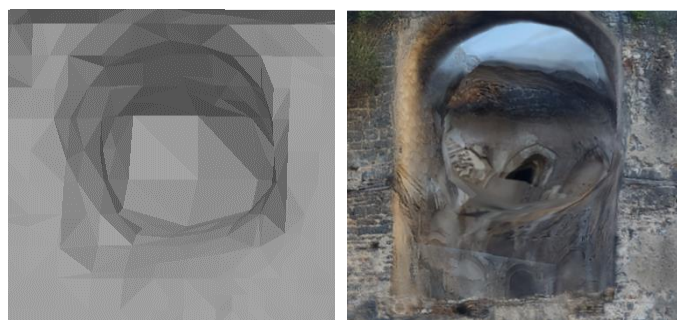
(a) Polygonal Shaded surface (b) Default Textured Surface Fig 2. Reconstruction for damaged portion of monument using photogrammetry:
