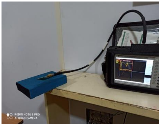
Testing on Anritsu VNA Master
