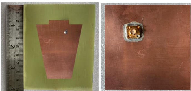
Fig.8. Printed antenna on FR4 with coaxial feed
