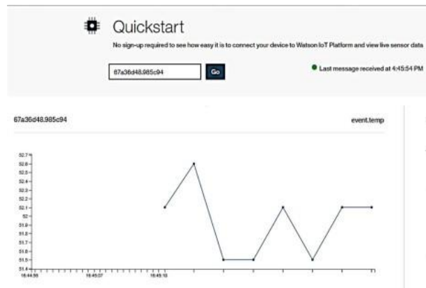
Figure 6: Quick-Start flow showing Raspberry pi processor temperature Vs time graph
