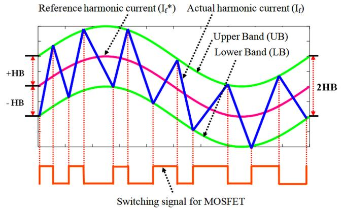
**Figure 3 Diagram of Hysteresis current controller**
