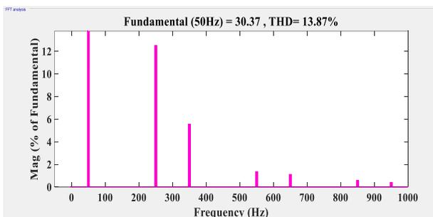
Figure 12 Harmonic analysis of  $I_{La}$  without using SAPF
