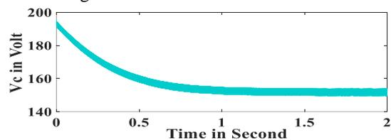
Figure 16 Variation of capacitor voltage  $V_c$  of SAPF w.r.t time
