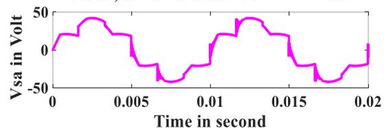
Figure 7 Variation of phase-a voltage of 3-phase source with  $R_s, L_s$  and non linear load w.r.t time
