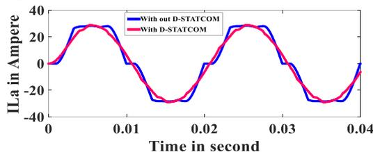
Figure 20 Comparison of waveform of ILa with and without SAPF
