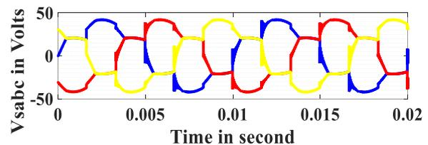
Figure 6 Variation of phase voltages ( $V_{sabc}$ ) of 3-phase source with  $R_s, L_s$  and non linear load w.r.t time
