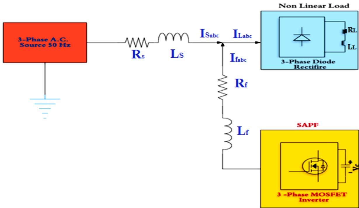
Figure 1 Structure of D-STATCOM as Shunt active power filter (SAPF)
