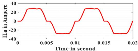
Figure 11 Variation of phase-a load current ( $I_{La}$ ) of non-linear load w.r.t time without using SAPF (taking into account source  $R_s$  &  $L_s$ )
