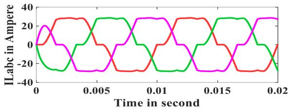
Figure 10 Variation of load currents ( $I_{Labc}$ ) of non-linear load w.r.t time without using SAPF (taking into account source  $R_s$  &  $L_s$ )
