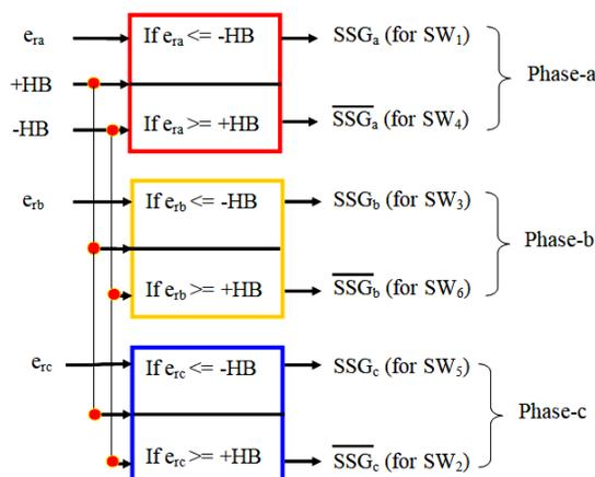
Figure 5 Generation of switching signals for MOSFET
