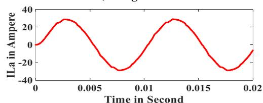
Figure 18 Variation of phase-a load current ( $I_{La}$ ) of nonlinear load w.r.t time with SAPF (taking into account source  $R_s$  &  $L_s$ )
