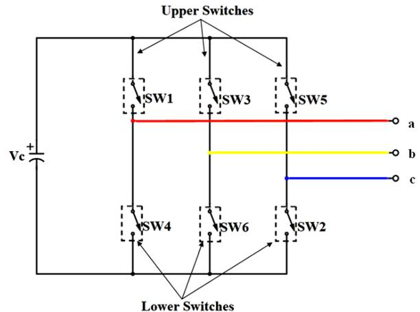
**Figure 4 Configuration of 3-phase MOSFET inverter**
