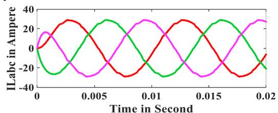
Figure 17 Variation of load currents ( $I_{Labc}$ ) of non-linear load w.r.t time with SAPF (taking into account source  $R_s$  &  $L_s$ )
