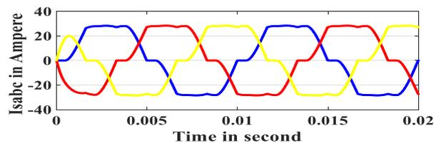
Figure 8 Variation of source currents ( $I_{sabc}$ ) of 3-phase source with  $R_s, L_s$  and non linear load w.r.t time
