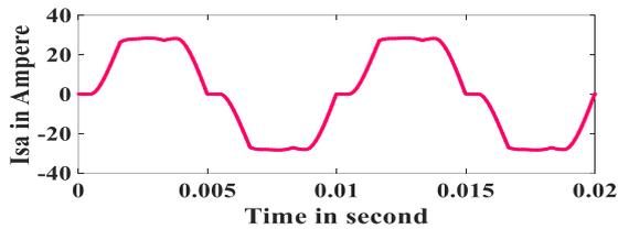
Figure 9 Variation of phase-a current of 3-phase source with  $R_s$ ,  $L_s$  and non linear load w.r.t time
