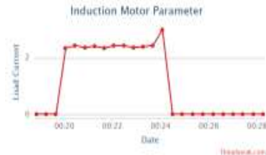
Figure 13 Fault Current Condition
