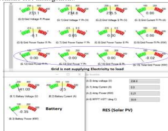
Fig.2.RES metering system while furnishing loads
