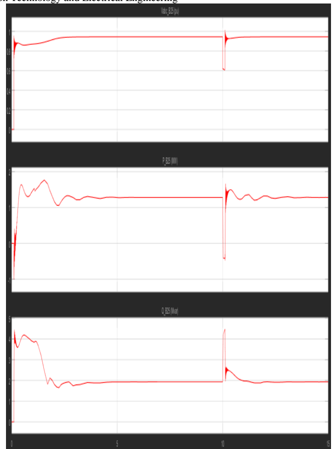
Figure 9. Output waveforms of with fault with SSSC
