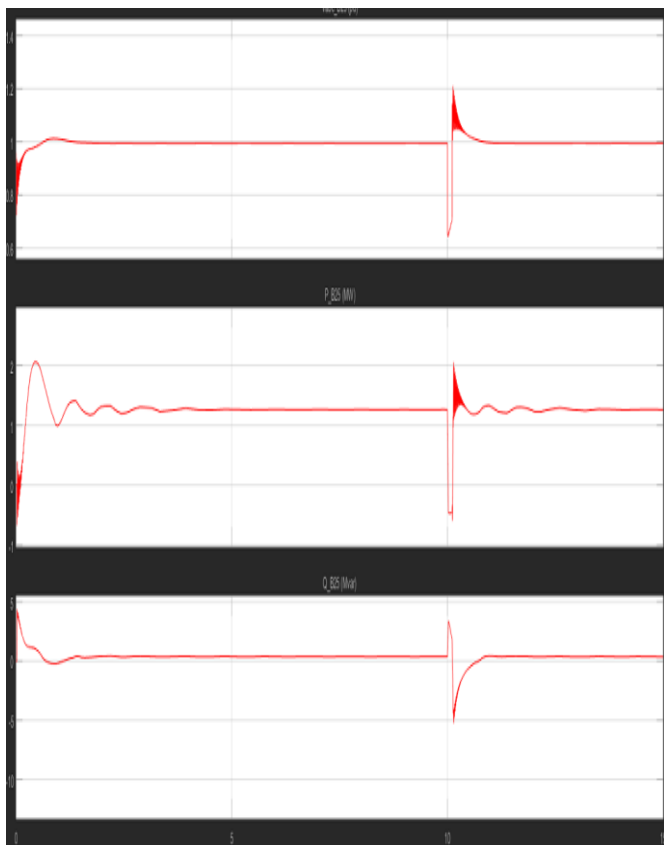
Figure 8. Output waveforms of with fault with SVC
