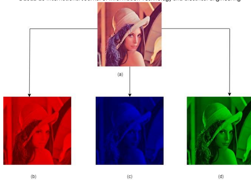
Fig 4.1 (a) Plain Image of “leena” (size 512 x 512), (b) Red plane from plain image, (c) Blue plain from plain image and (d) Green plain from plain image.
