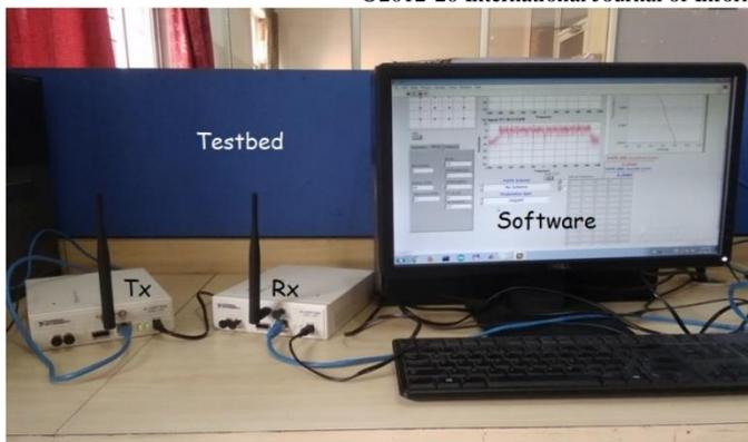
Figure-5: Test Bed with Software Defined Radio- NI USRP 2922
