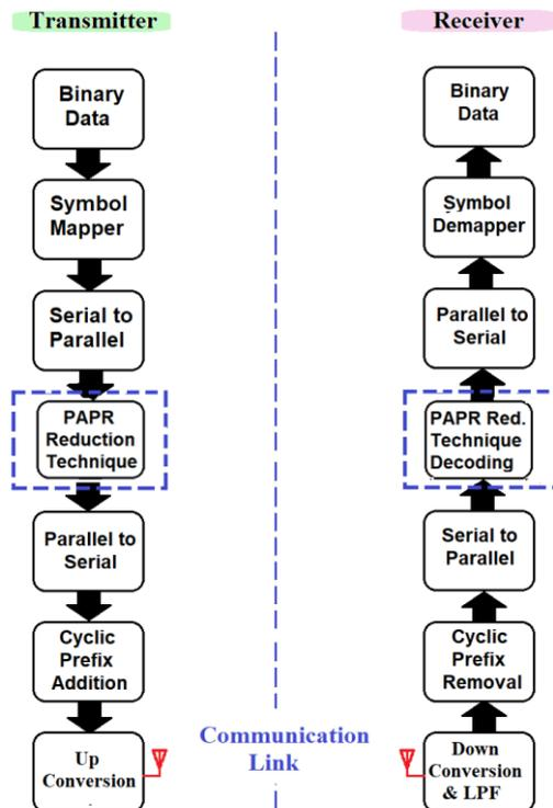
Figure-4: Block schematic of OFDM Transmitter and Receiver
