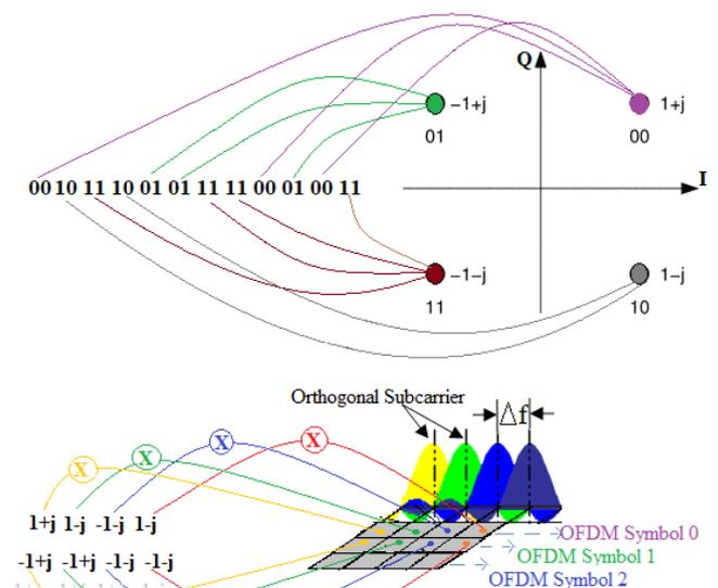
Figure-1: OFDM Symbol Formation for 4-QAM Scheme
